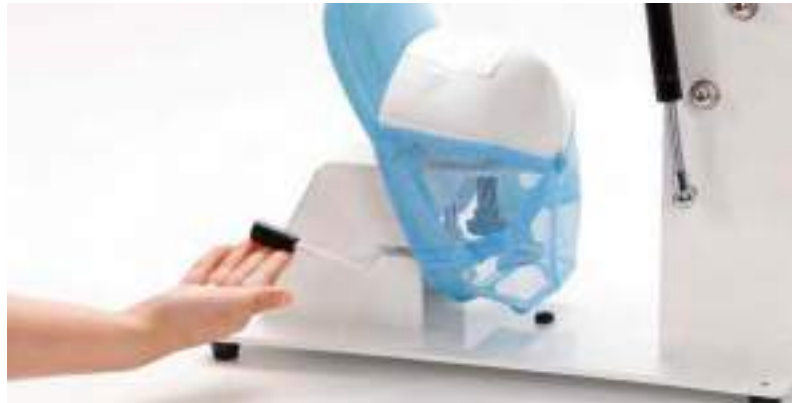
Holding Device It allows the cap to fit the pad for good printing results.
